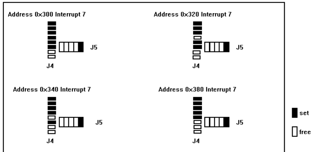
Figure 17: Jumper J4 - Address Setting
